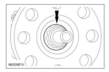
6. Using the Output Flange Remover, remove the output shaft flange.
