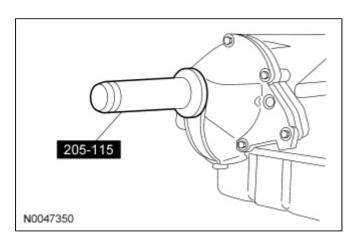
2. Using the Output Shaft Flange Installer and the Drive Pinion Flange Installer, install the output flange.
