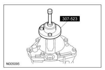
7. Using the Torque Converter Fluid Seal Remover and Slide Hammer, remove and discard the extension housing seal.
